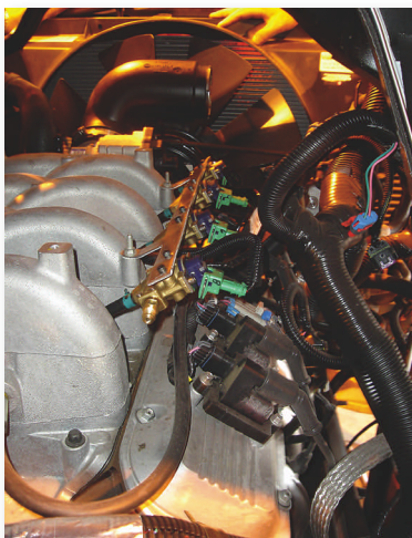
CleanFuel creates a dedicated propane-fueled GM 8.1L engine by replacing only the gasoline tank, fuel pump and injector rails with an OEM-compatible propane fuel system.
