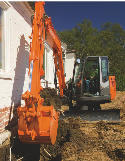
The swing boom on the Hitachi ZX85USB-3 excavator enables digging parallel to walls with an "ultra-short-swing" machine that's still sized at 8.5 metric tons. That is beyond the official mini-excavator size, but in a range many manufacturers still define as compact.
